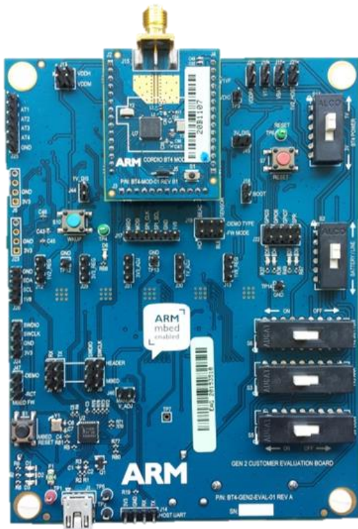
Figure 2.1a – Gen 2, BT4 Eval Board, Top Side
